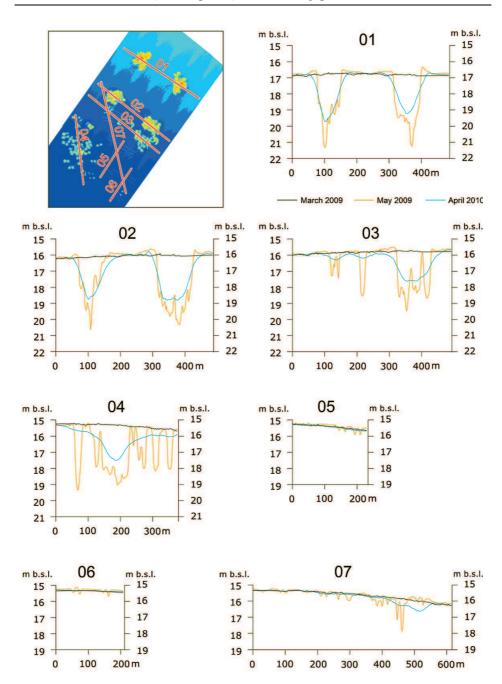
**Figure 14.** Morphological profiles across dredging pits formed by planned stationary dredging (Profiles 01 and 02), exploited by unplanned stationary dredging (Profiles 03 and 04), and morphological profiles across furrows left by trailer suction dredging (Profiles 05, 06 and 07)
