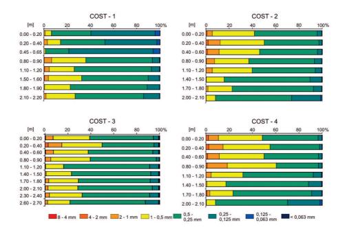
Figure 5. Grain size distribution of deposits in cores COST-1, 2, 3, 4
