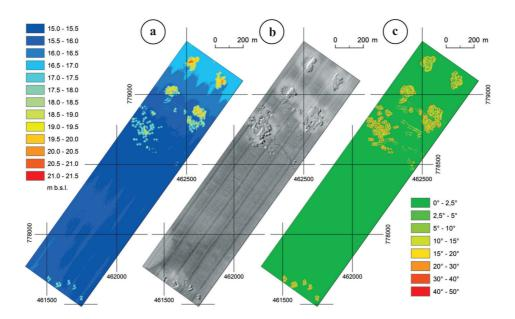
Figure 8. Area of investigation directly after sand extraction (May 2009): a) bathymetric map of the sea bottom; b) sonar mosaic of the sea bottom; c) gradient of slopes of dredging pits and furrows
