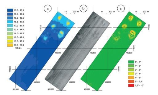
Figure 9. Area of investigation 11 months after sand extraction (April 2010): a) bathymetric map of the sea bottom; b) sonar mosaic of the sea bottom; c) gradient of slopes of the dredging pits and furrows
