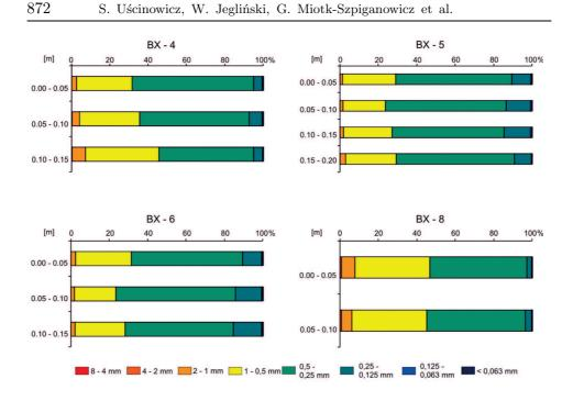
Figure 11. Grain size distribution of sediments between the dredging pits 11 months after extraction ceased
