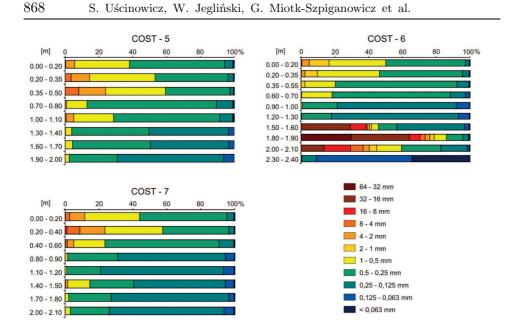
Figure 6. Grain size distribution of deposits in cores COST-5, 6 and 7
