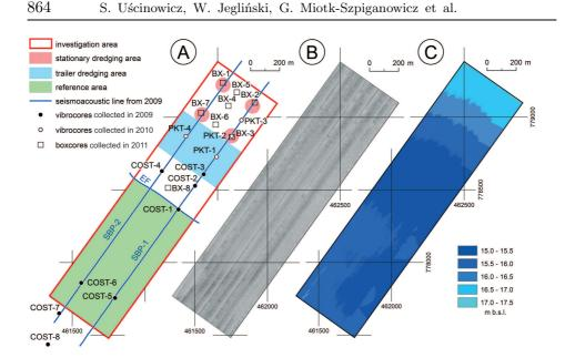
**Figure 2.** The area of investigation directly before sand extraction (March 2009): a) plan of the test field; b) sonar mosaic of the sea bottom; c) bathymetric map of the sea bottom
