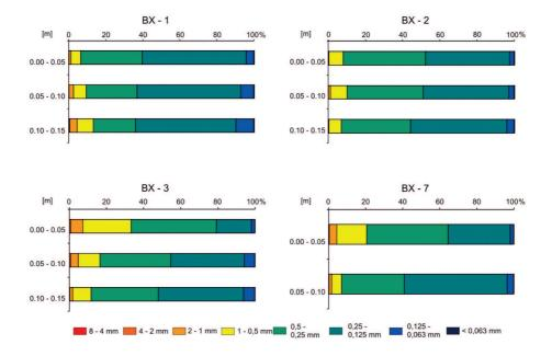
Figure 10. Grain size distribution of sediments filling the dredging pits 11 months after extraction ceased
