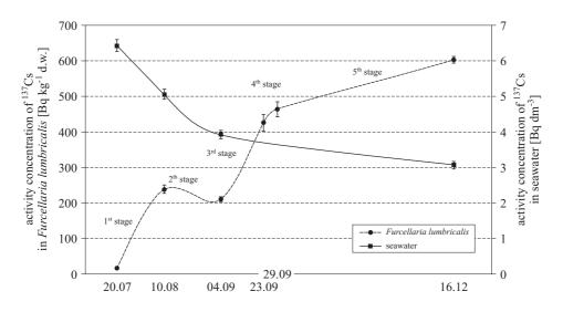
Figure 6. Plots showing the changes in concentrations of  $^{137}$ Cs in *Furcellaria lumbricalis* and in seawater recorded during exposure from 20 July to 16 December
