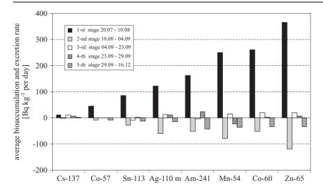
**Figure 7.** Bioaccumulation and excretion rates calculated for five exposure periods for <sup>54</sup>Mn, <sup>60</sup>Co, <sup>65</sup>Zn, <sup>113</sup>Sn, <sup>57</sup>Co, <sup>241</sup>Am, <sup>110m</sup>Ag and <sup>137</sup>Cs
