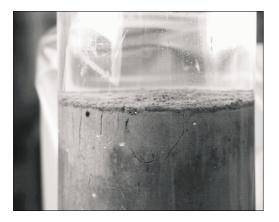
Fig. 2. Photograph of a sediment core from the central Kattegat showing the intact fluffy layer on top of the sandy sediment
