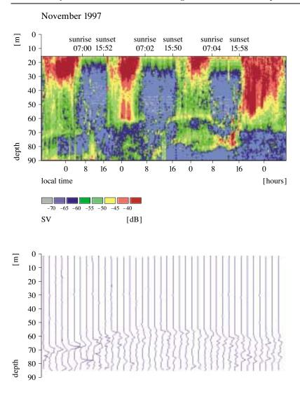
Fig. 6. 3.5 day condensed echogram (upper), vertical profiles of density gradient calculated for different instants of observation (lower) in November 1997
